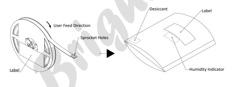
1. Moisture-sensitive product is packed in a dry bag containing desiccant and a humidity card according JEDEC-STD-033.
